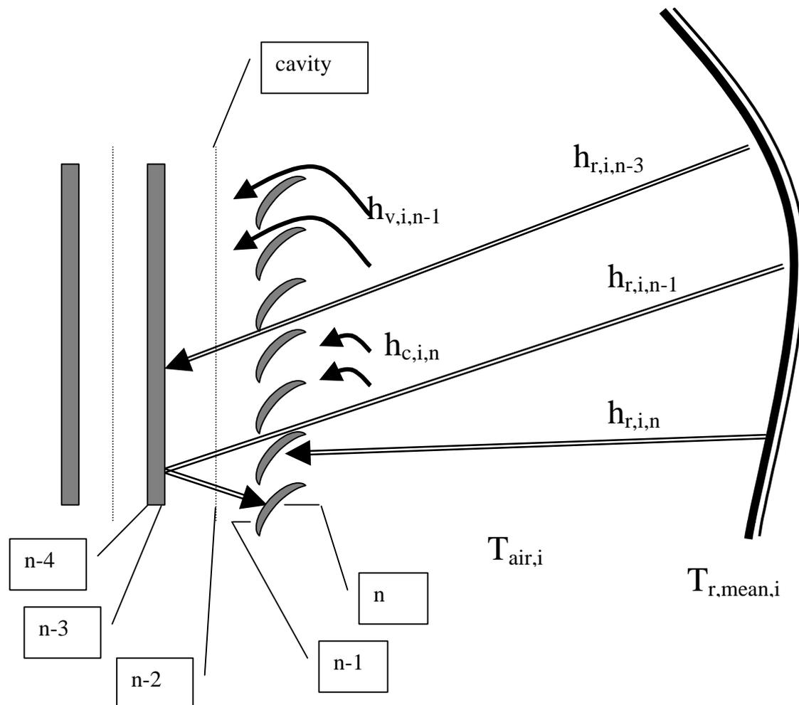
Heat is exchanged by convection, thermal radiation and ventilation from the indoor environment to the window/façade.
