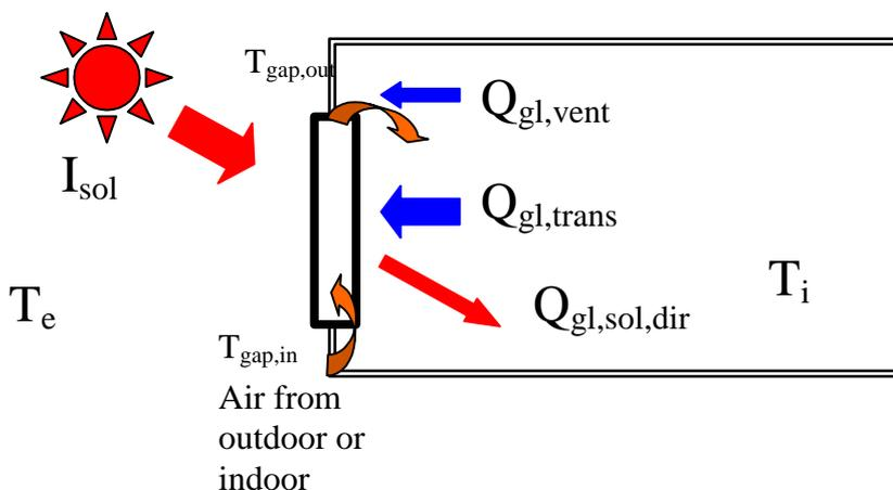
We use the symbol  $g_l$  (“glazing”) for the window or façade, because we concentrate on the transparent (“glazed”) part of the system.
